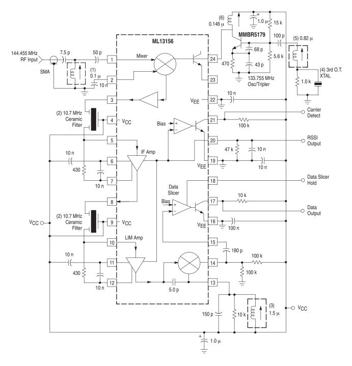
NOTES: 1. 0.1  $\mu\text{H}$  Variable Shielded Inductor: Coilcraft part # M1283–A or equivalent.
