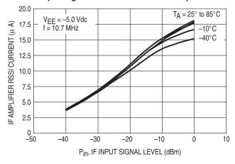
Figure 7. Limiter Amplifier RSSI Output Current versus Input Signal Level and Temperature
