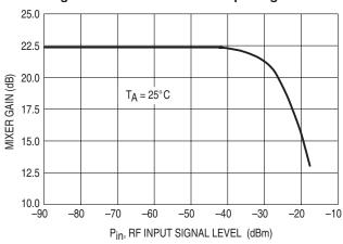
Figure 5. IF Amplifier Gain versus Input Signal Level and Ambient Temperature
