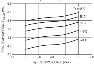
Figure 3. Drain Currents versus Supply Voltage
