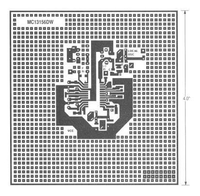
Figure 33. Ground Side View
